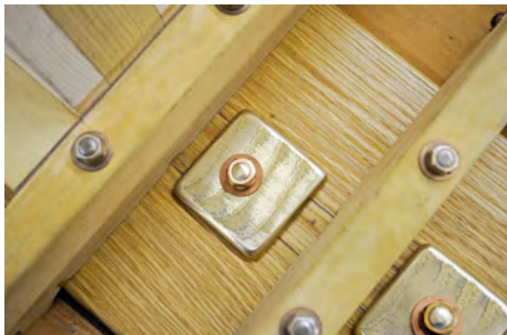
Figure 24) Bronze pads that were used in BEN's last refit at Ballentine's and were replaced and enlarged with this restoration. (Fields)
