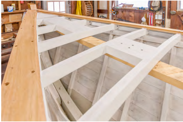
Figure 18) Deck beams are built in White Oak. They were then covered with pine and canvas as in the original plans. (Fields)
