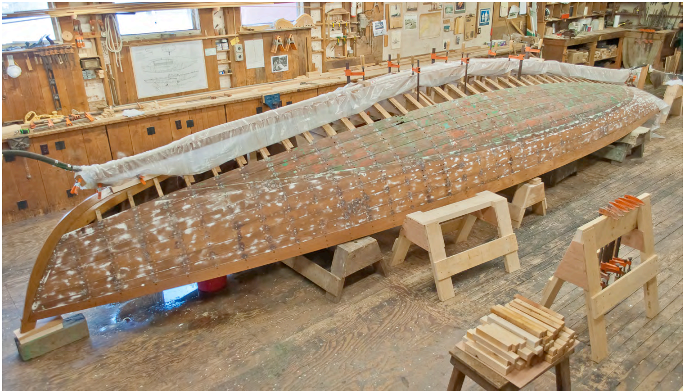
Figure 17) A new Keelson is fit then steamed in place. (Fields)
