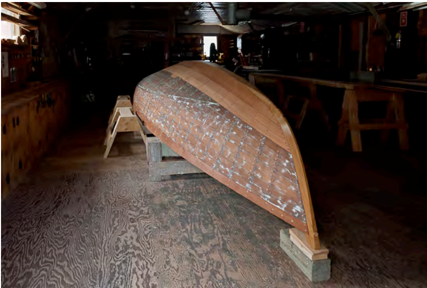
Figure 13) Much of her original mahogany planking was suitable to be reused. However, the garboard and broad planks were replaced. (Fields)
