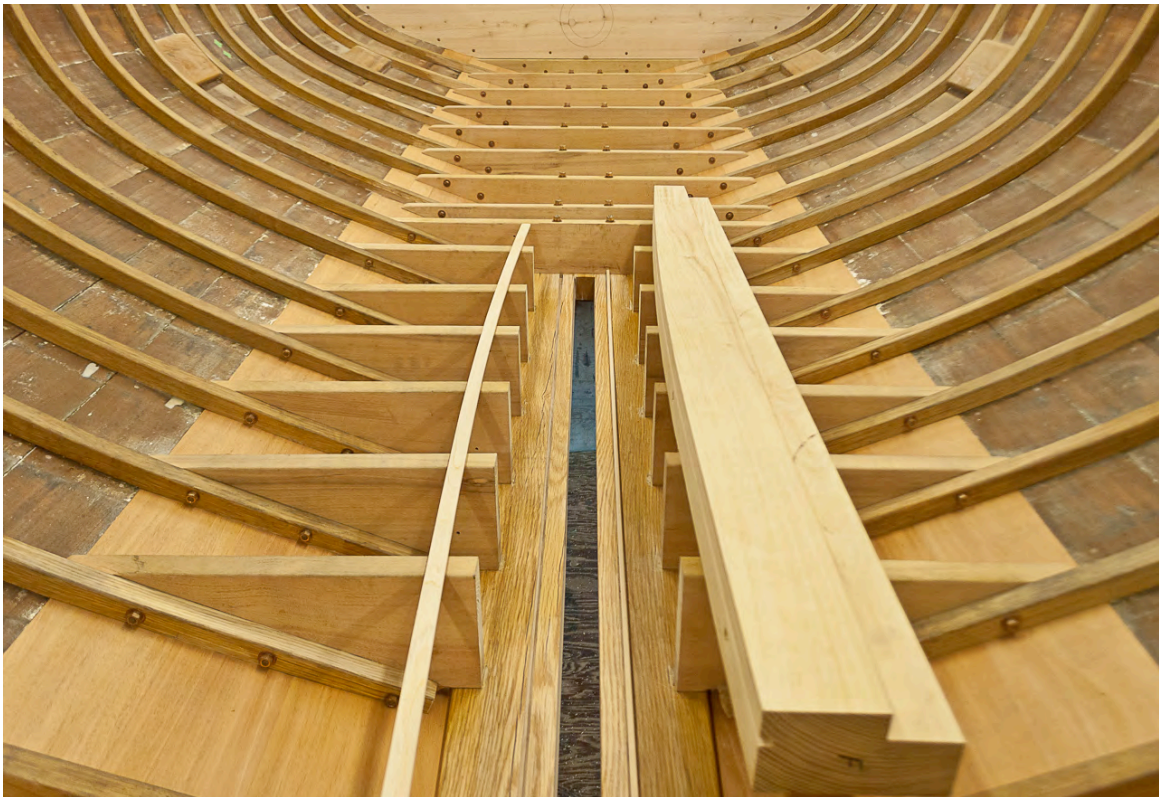
Figure 22) Centerboard log is in locust and is splined with a strip of cedar that is also splined into the keelson.
