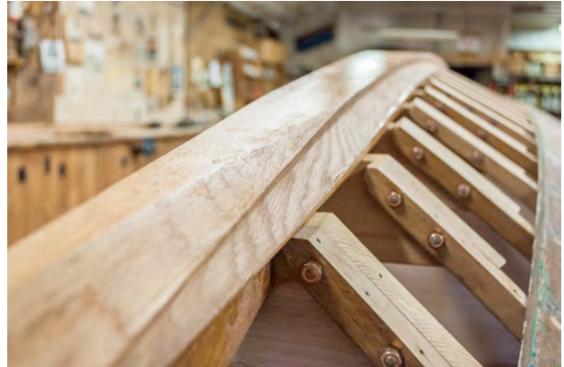
Figure 16) The White Oak keelson steamed and fastened in place. (Fields)
