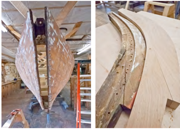
Figure 6) Restoration is underway, the majority of this mahogany planking we were able to reuse. The stem was removed and replaced as to the plans and from recreating the original. (ABS)
