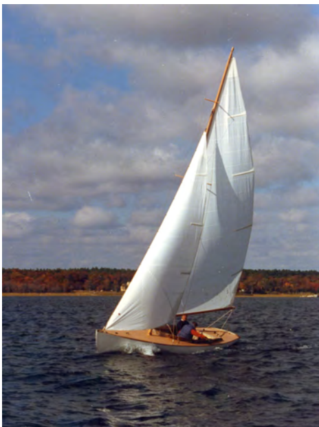
Figure 5) Bill Harding sailing BEN (perhaps with Roger Taylor). She is tested with different sails and rig modifications. The headstay is brought well forward and this jib is much larger than the one ultimately decided on. (Harding)
