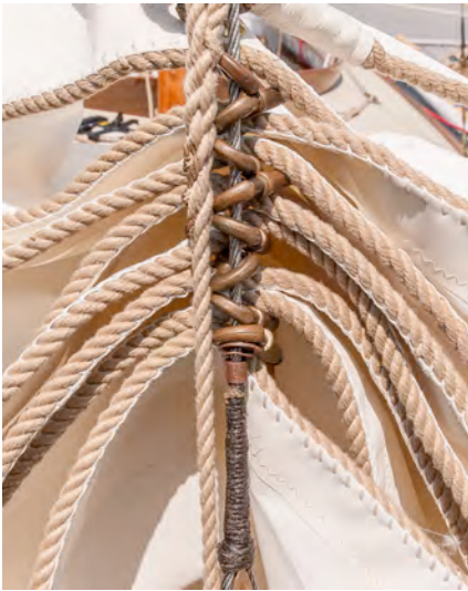
Figure 27) The jib features a hand sewn bolt rope in Posh 3 strand. The bronze hardware is period. The headstay was hand seized and tarred as originally done. (Fields)
