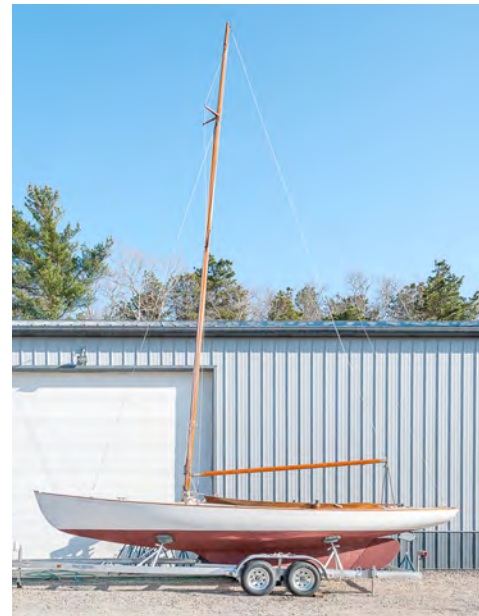
Figure 9) The rig on BEN is more raked than the position established for the Stuart Knockabout. (Fields)
