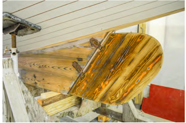
Figure 12) The Yellow Pine deadwood and rudder are in great shape and are reused. Here the deadwood is getting fit and fastened to the keelson and the rudder hung. (Fields)
