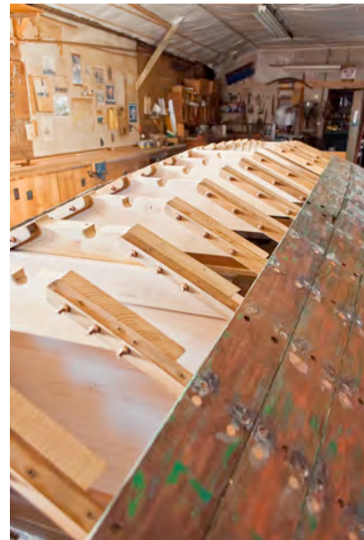
Figure 21) Rounded edges and ends are sealed and help to keep water from wicking into the grain, combating decay. (Fields)
