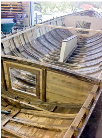
Figure 19) Looking forward in BEN before her restoration. All frames were sistered as most of the originals were cracked. (ABS)
