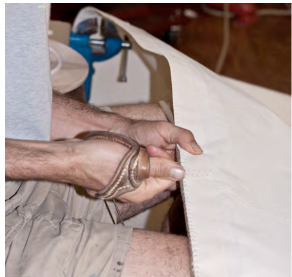
Figure 25) The sails, although made with the modern material of Dacron, are built traditionally with hand sewn bolt rope, narrow panels and cream color. (ABS)
