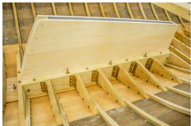
Figure 23) Custom angles are cast in Bronze to fortify the area around the centerboard. Splined pine makes up the trunk sides and is lapped into the Locust centerboard log. (Fields)
