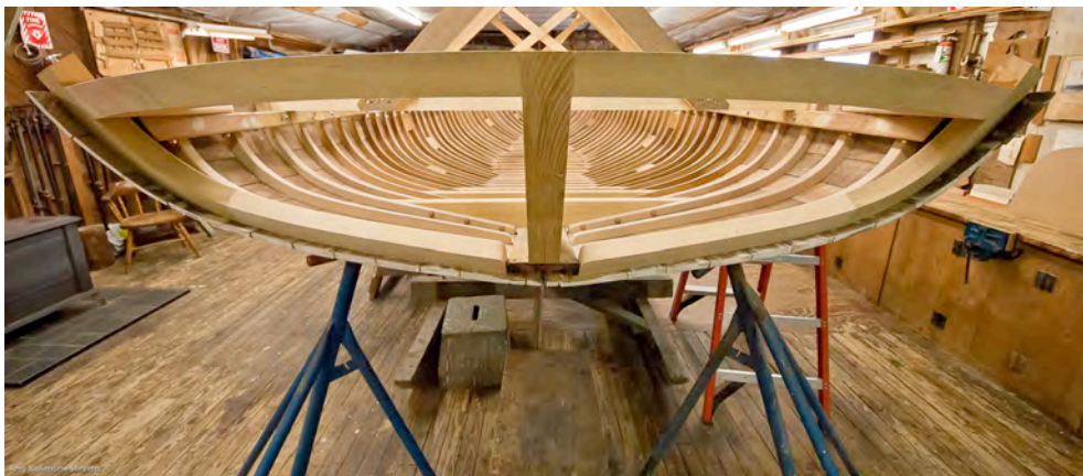
Figure 26) The transom frames are in place as well as the stern knee which now is consistent with the plans. The quarter knees are notched in place. (ABS)
