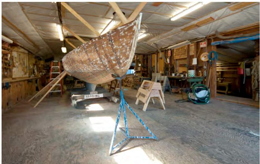
Figure 11) BEN's rebuild is underway, bracing and templates are used to re-establish her port and starboard symmetry and shape. (ABS)
